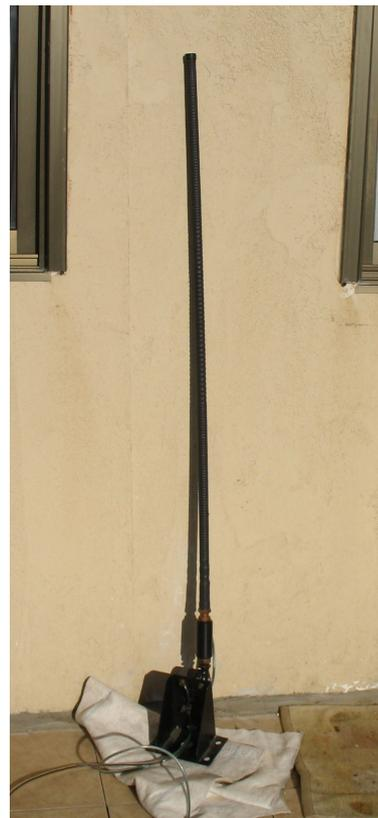
**Figure 6** NVIS-HF1-BC antenna. The antenna height is 1.5m.
