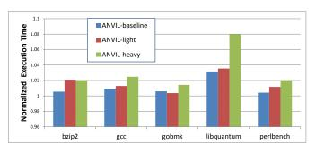
Figure 4: Sensitivity of Execution Overheads to Potential Future Attacks: The figure compares normalized execution times for selected benchmarks running on ANVIL-enabled system with three configurations. *ANVIL-Heavy* is configured to have the highest sampling rate while *ANVIL-Light* has the lowest last-level cache miss threshold.
