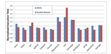
**Figure 3: ANVIL's Impact on Non-Malicious Programs:** The Figure shows execution times for selected benchmarks on ANVIL-enabled system and a system with doubled DRAM refresh rate. The values shown are normalized to execution time without ANVIL and at a single refresh period.
